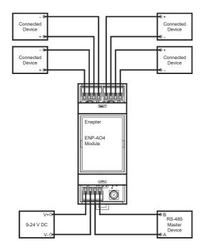
Note: 1 Amp Circuit Breaker recommended to use on power line for the ENP-AO4 Module.
