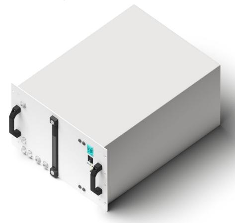
Enapter's Water Tank provides storage for 38 litres of clean water for the AEM Electrolyser. The water tank is rack mountable into a standard 19" cabinet. The tank contains a conductivity sensor and a pump system to supply up to 11 AEM Electrolysers with clean water.
